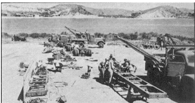
In new Caledonia, 1942, ordnancemen assemble vehicles which have arrived crated in sections. By October, 25 men would complete six vehicles a day on this assembly line.
